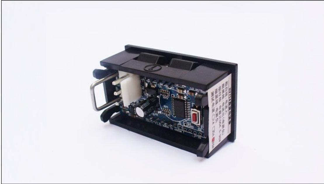
Ammeter with isolated power supply
